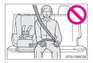
A child seat is attached to the rear right seat Please do not sit in the rear center seat when you get rid of it. when. Seat belts and child seats Can interfere and the seat belt can be worn correctly Serious scratches in the event of a sudden brake or collision Harmful or, in the worst case, death There is a risk of
