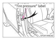
The specified air pressure of the tire is the tire on the driver's side. You can check it on the pneumatic label.
