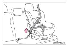
Seat belt on child seat Install and buckle the plate Insert until you hear a "click" Include. The belt is not twisted To do it.
